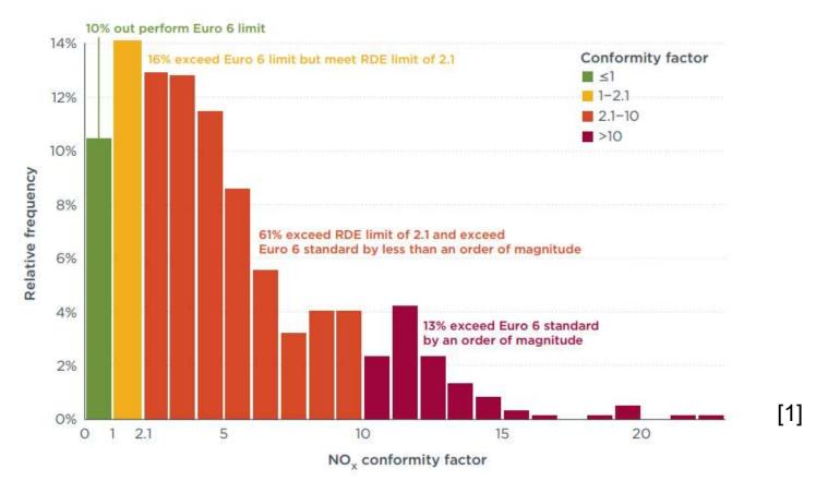
Dieselgate exposed discrepancy between lab tested emissions and real drive emissions
