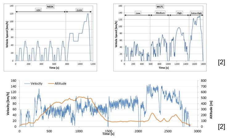
Transient nature of real drive cycle not represented under test conditions including WLTC
